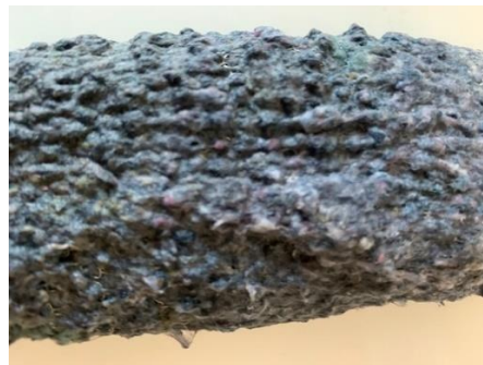
Photo Above is a close-up view of a used Lint Catcher that has protected your plumbing from excess lint entering the home's sewer pipe. When a lint catcher is full of lint, replace it.
